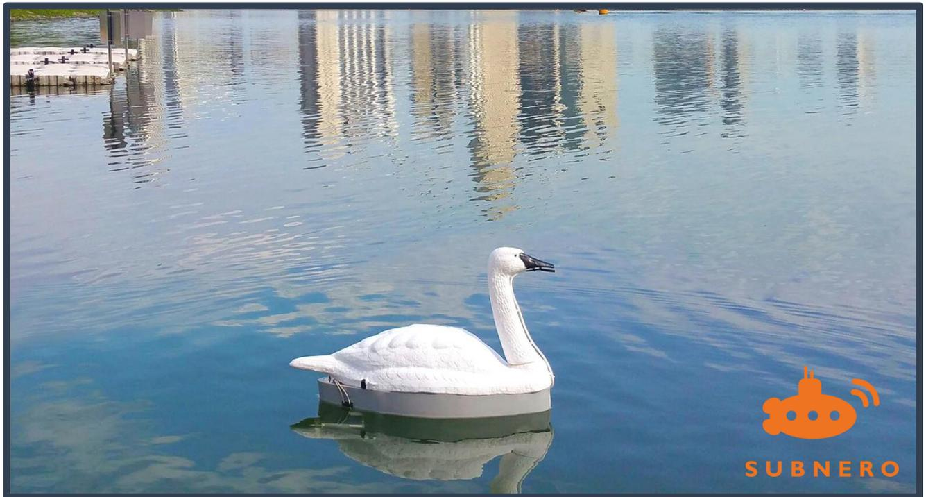
**SWAN:** Autonomous, intelligent, cloud-based networked system for real-time water quality measurements and monitoring
