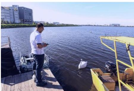
The autonomous SWAN robot monitors water quality parameters while navigating the water surface. A centralized cloud server collects the water quality data transmitted by the SWAN robots and other water assets and displays data in real-time on a web interface. Users can access the data from diverse platforms, including tablets and mobile phones.
